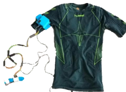
Figure 2: Suit fitted with dielectric electro-active polymer
